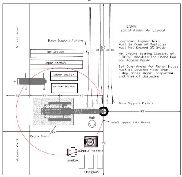
Figure 10: Typical Site Component Layout before Rotor Assembly. Grade area shown in figure is absolute minimum.
